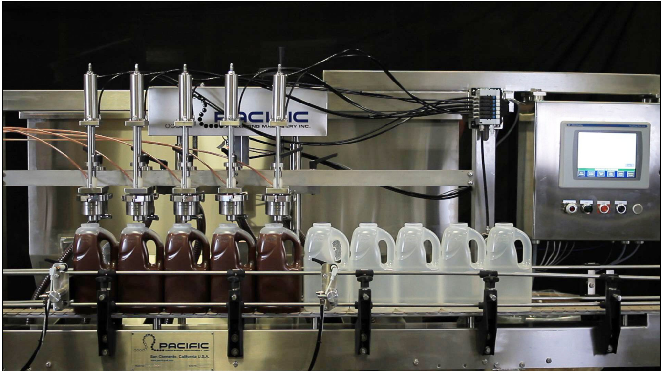
Pacific 5-Station Volumetric Pump Filling Machine for 64 and 128-ounce Sauces at 25 Gallons per Minute
