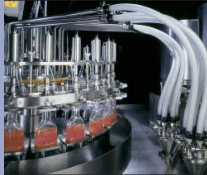
24-station two-stage pourable salad dressing filling machine
