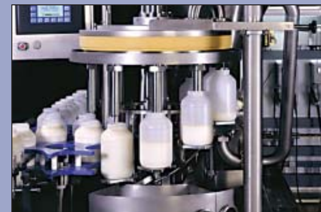
10-station gallon filler for viscous products at 100 containers per minute
