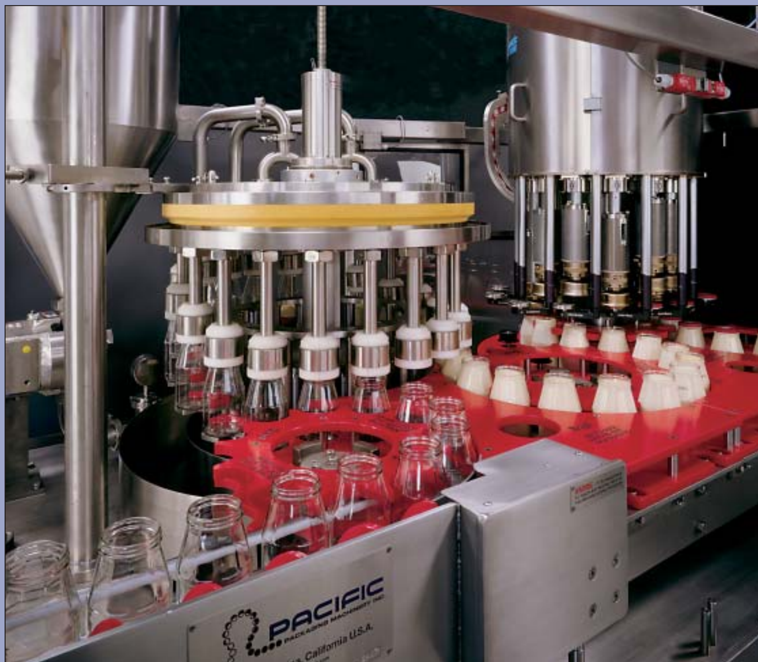
Monoblock 20-station filling turret and 12-station capping turret for viscous products. Capable of speeds up to 400 containers per minute
