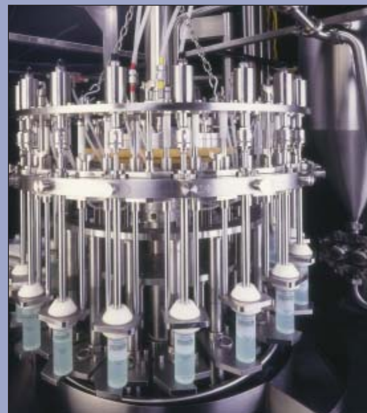
18-station personal care filling machine for viscous products at 275 containers per minute
