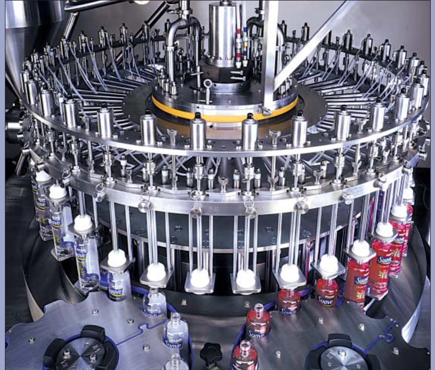
A 36-station personal care filler proven at 500 container per minute filling capacity
