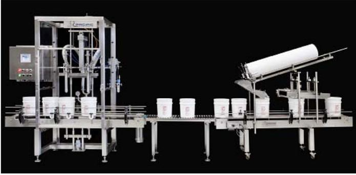
The two-station or four-station fully automatic filling and lidding system provides a bottom-up fill that is ideal for a wide variety of thin, foamy and viscous products.
