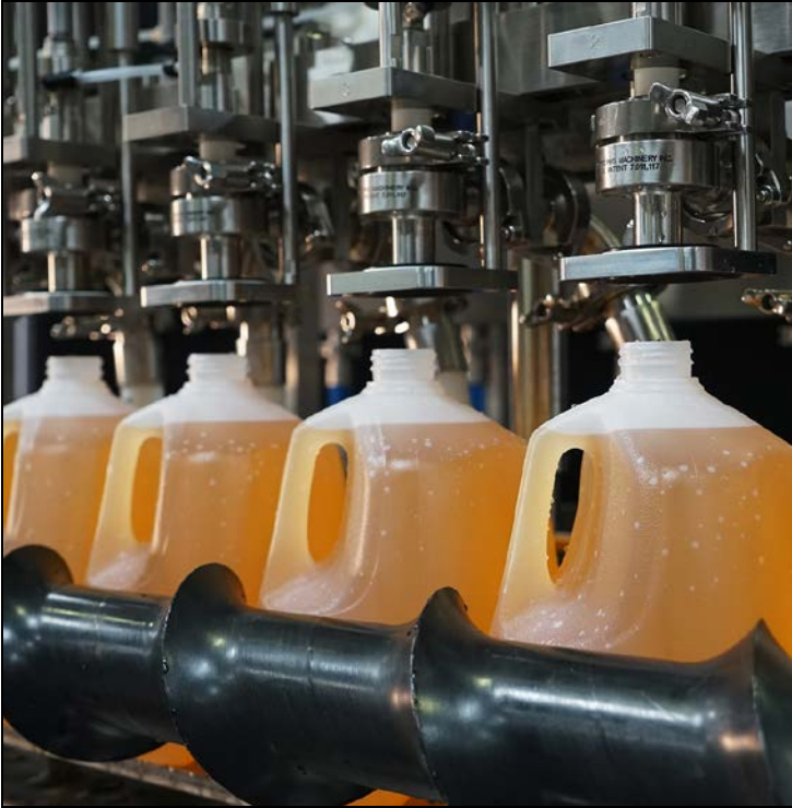
Pacific 6-Station Volumetric Pump Filling Machine and 128-ounce containers at 20 Gallons per Minute
