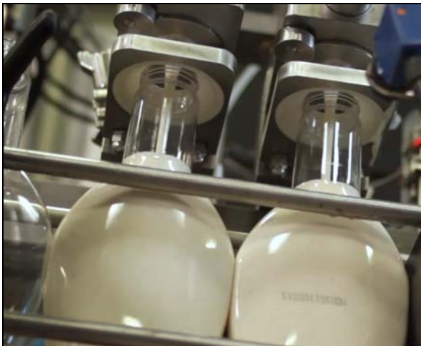
Pacific 4/2-Station Volumetric Pump Filling Machine for Single and Two-Phase Salad Dressing Products
