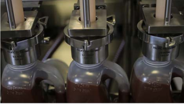
Pacific 5-Station Volumetric Pump Filling Machine for 64 and 128-ounce Containers at 25 Gallons per Minute
